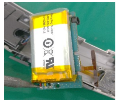
Remove battery wire.
