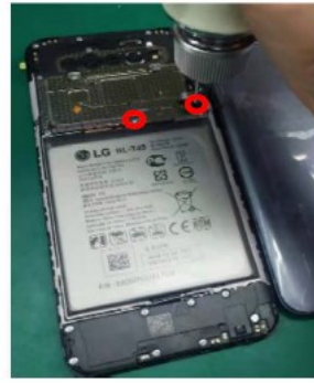
7. Disassemble Connector (9 ea)
