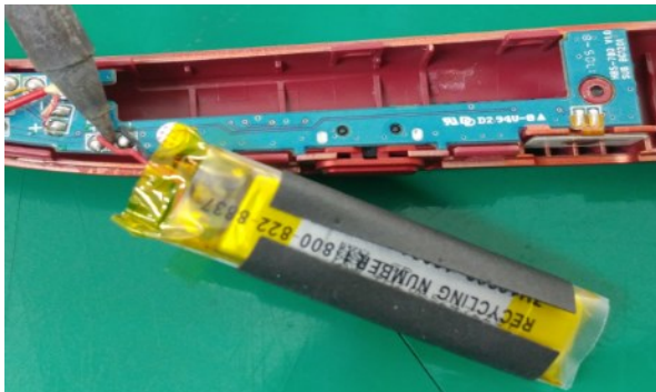
Remove battery wire.
