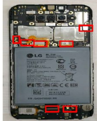
7. Disassemble Connector (9 ea)
