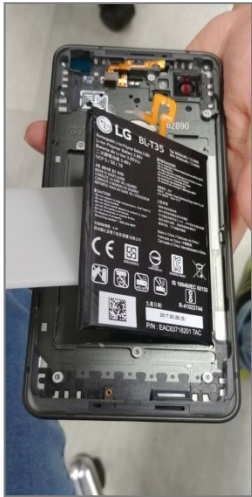
17. Lifts up the battery using the hera
