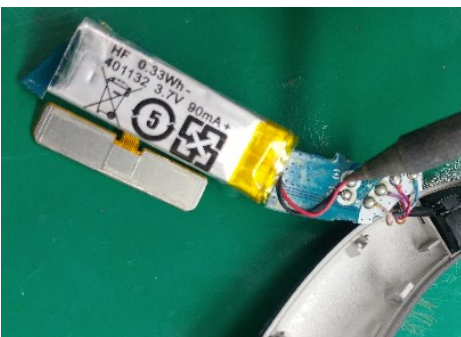
Remove battery wire.
