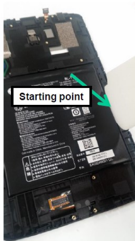
Disassemble battery pack by tool. (The principle of the lever)
