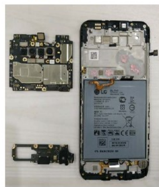
8. Disassemble main PCBA and Sub PCBA
