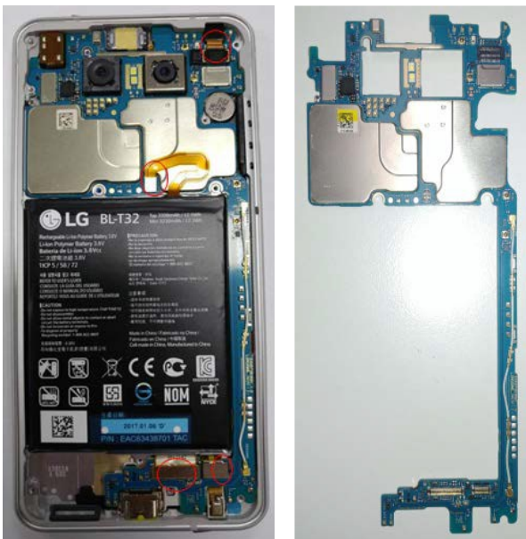
7. Disconnect 4 connectors / main PCB
