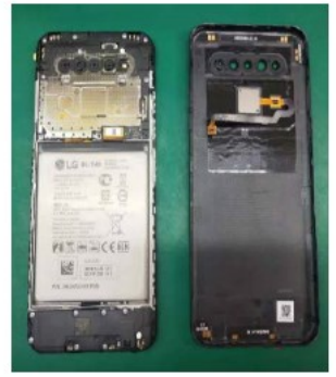
8. Disassemble main PCBA and Sub PCBA
